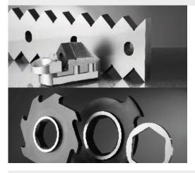
SIKNIVES for shredding are manufactured from the new generation of steel alloys with different hardening processes (through-hardened, case-hardened, nitrided, etc.) and heat treated in vacuum to maximise blade performance.
